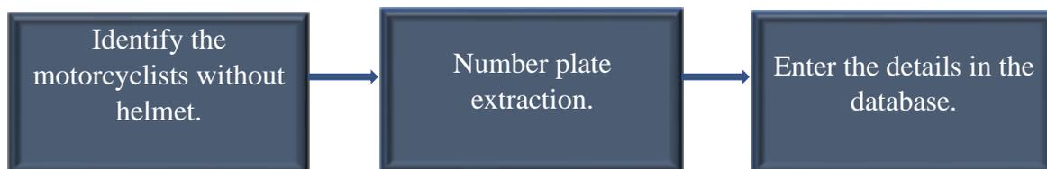
Pearl aims to help the concerned authorities identify motorcyclists without helmet. A video camera installed on the road provides input to the system. The helmet detection system does the following:
