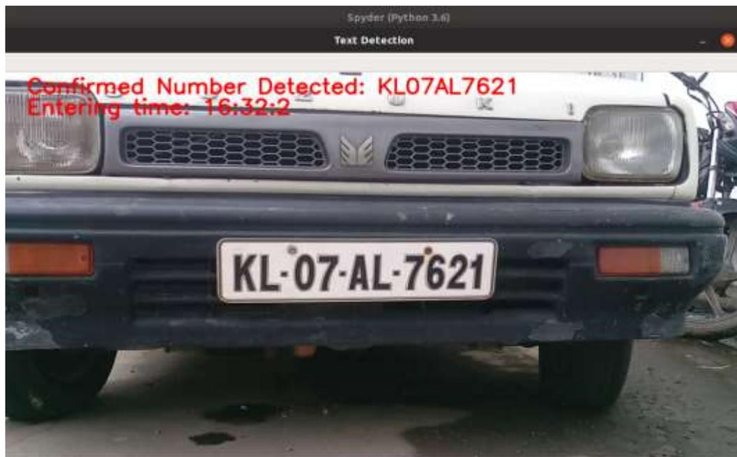
*Figure 2: Vehicle Registration Number Detection*
